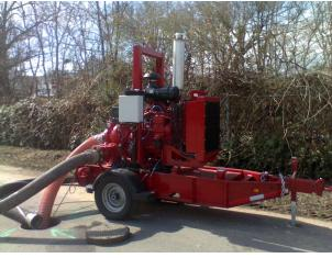
As an MWI Pump Partner, we are proud to offer the PrimeRite™ CT004. It is a perfect choice for contractors, mining operators, and general industrial or municipal use. With flow rates up to 1100 GPM and solids handling to 1 1/2", the CT004 is great for your temporary pumping needs!
