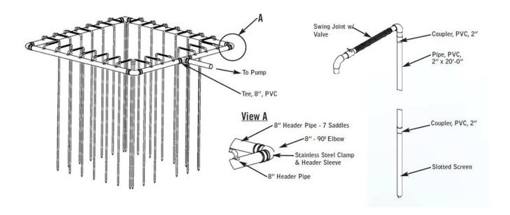
The wellpoint system is used to lower the water table to allow construction of buildings and civil works. All pipes shown bring water from the ground to the suction port in the pump. Discharge from the pump is then either directed to a canal or catch basin depending on site conditions.
