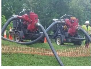
WMS is proud to offer the AmeriPumps WP 150/200 Automatic Priming Centrifugal Pump. It excels in well-point dewatering, straight dewatering, and sewer bypass, making is one of the most versatile pumps available. It also has the Sykes Univac vacuum system that allows the pump to prime and re-prime automatically, operate with the suction intake intermittently exposed to atmosphere, and to run dry for indefinite periods of time without harming
